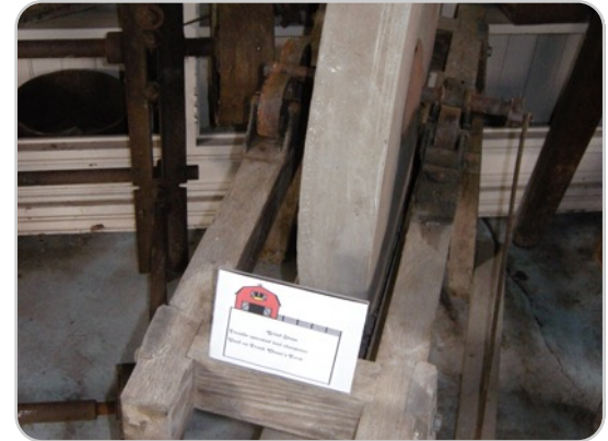
Grind Stone: treadle operated tool sharpener. Used on Frank Chase's Farm.
